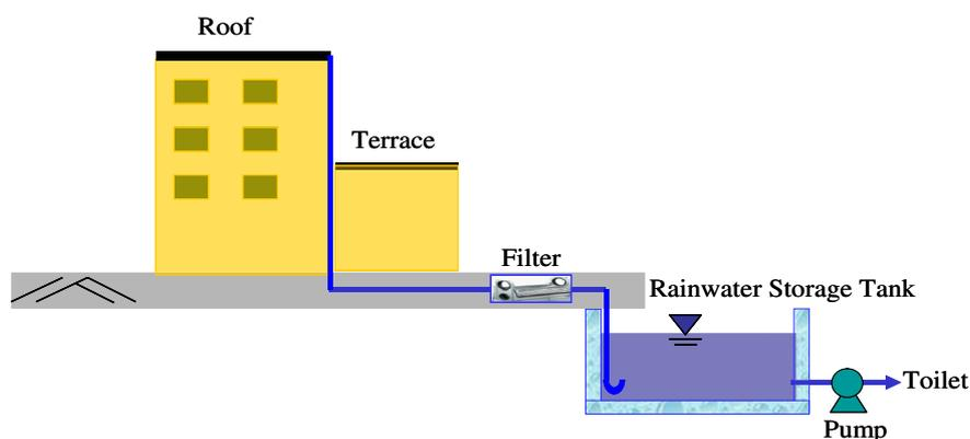
**Fig. 2 – Schematic diagram of Rooftop RWH system.**
