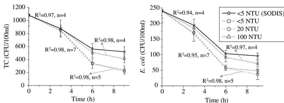
**Fig. 8 – Effects of different initial turbidity values on microbial inactivation with time for neutral pH rainwater under weak weather conditions.**
