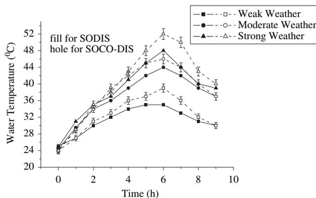
**Fig. 4 – Water temperature comparison between SODIS and SOCO-DIS system under different weather conditions.**
