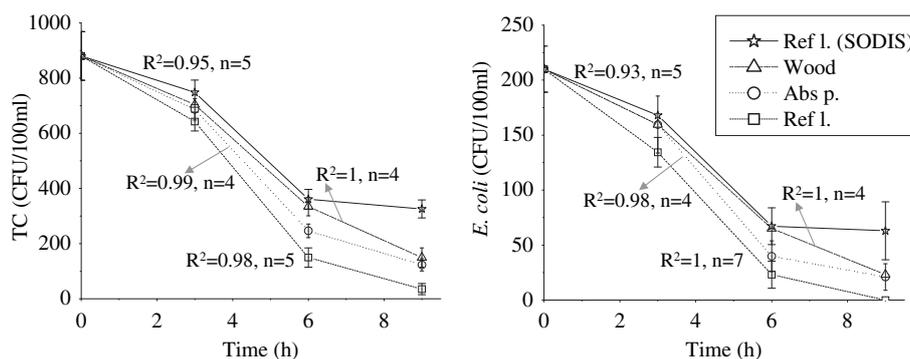
**Fig. 5 – Microbial inactivation with different base surfaces of solar collector with low turbidity (5NTU) and neutral pH values under moderate weather conditions.**
