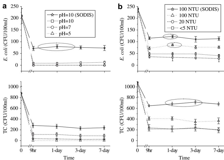
Fig. 9 – Microbial re-growths for different initial; (a) pH values under moderate sunlight with low turbidity (5NTU), and (b) turbidity values under weak sunlight with neutral pH.
