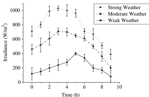
**Fig. 3 – Irradiance changes with exposure time under different weather conditions.**
