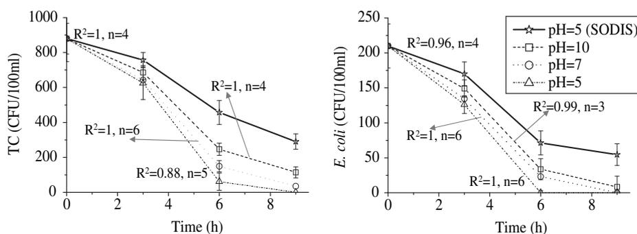
**Fig. 7 – Effects of different initial pH values on microbial inactivation with time for low turbidity (5NTU) rainwater under moderate weather conditions.**
