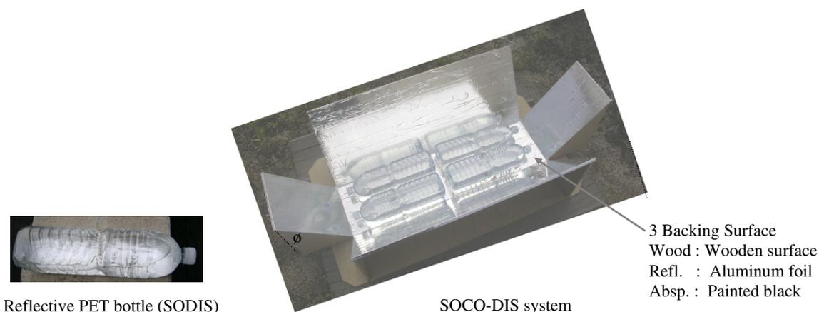
**Fig. 1 – Rainwater samples in PET bottles kept directly at rooftop for SODIS and inside collector for SOCO-DIS system.**
