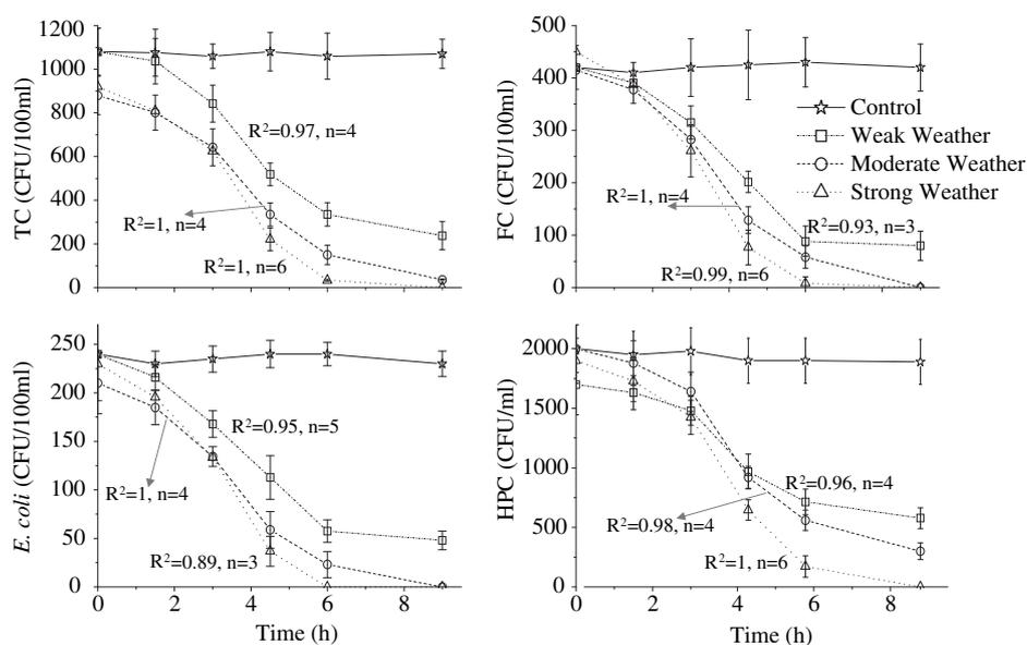
**Fig. 6 – Microbial inactivation in SOCO-DIS system under different weather conditions with low turbidity (5NTU) and neutral pH values.**
