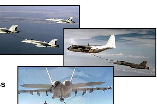
Every F/A-18E/F is capable of serving as an in-flight refueling tanker
